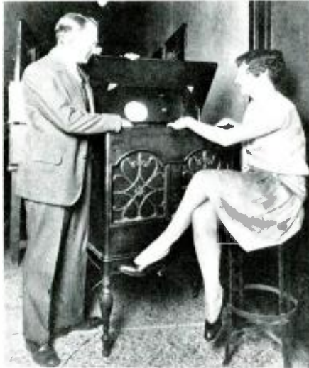
A 1929 Westinghouse tv set, above, being demonstrated by famed tv inventor Vladimir Zworykin, who later worked for RCA. (He invented the iconoscope.) Picture is projected from a mirror. In late 40s, "Uncle Milt" Berle, performing in outrageous costumes, dominated video and won the name, "Mr. Television."
